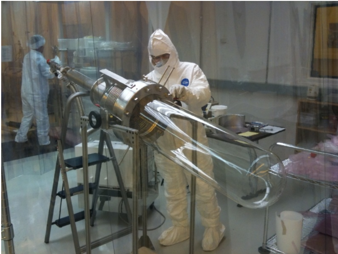
Figure 5-1: COUPP-60 Inner Vessel under assembly in clean room.
